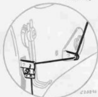
Fig. 8. Threading Needle Thread Take-up
